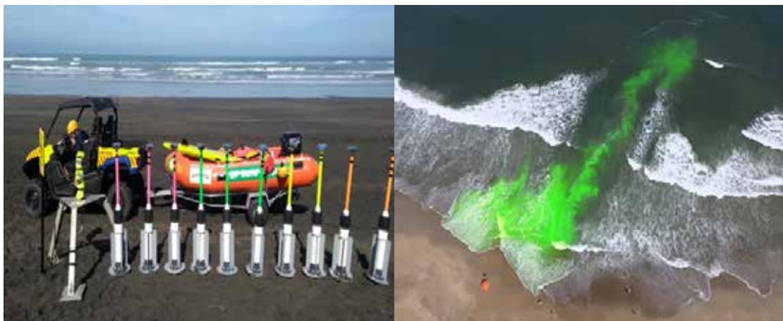
Figure 5: GPS drifter and dye used to study and identify rip currents in the field. Source: Rip current CMAR, presentation 2020.
